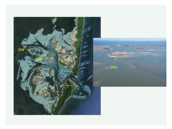
Figure 5. Dredged material placement islands, 26A and 26B, which have historically been used for disposal of material from the Oyster Creek channel but have become environmentally sensitive due to habitat establishment.
