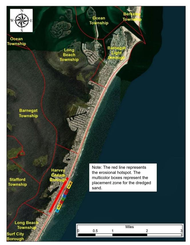
Figure 6. Location for the construction of the nearshore placement site at the southern half of Harvey Cedars, NJ.
