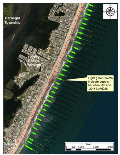
Figure 5. Profile lines at Harvey Cedars, showing depth zone from -10 to -20 ft NAVD88
