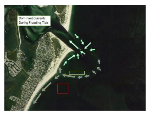
Figure 3. Current placement areas for dredging of Barnegat Inlet for routine maintenance dredging conducted twice per year. Red box is preferred, just outside of ebb shoal/nodal point and should be utilized as much as possible. Yellow box is used when placement operations are limited during higher sea conditions.
